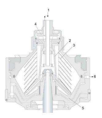
Fig. 1. Typical bowl drawing for a solids-ejecting centrifuge in clarifier execution. Drawing details do not necessarily correspond to the centrifuge described.
